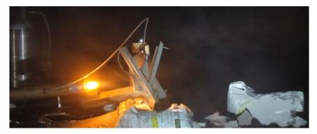
The solution to this issue was the addition of a heavy concrete slab over the base of the test stand, which also acted as a much better blast deflector. No other rapid test stand configuration changes have occurred since this incident.
